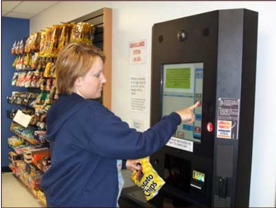
When customers bring their purchases to the kiosk, an interrogator reads the tags and tallies up the total sale. The patrons can then pay with cash or a credit card.
